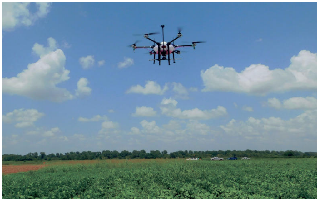
UAV USED TO APPLY HERBICIDES. This image shows a UAV/drone applying herbicides to a research field at Texas A&M University. The system is equipped with a four-nozzle boom and has a capacity of over five quarts. Photo courtesy of Texas A&M Weed Science.
