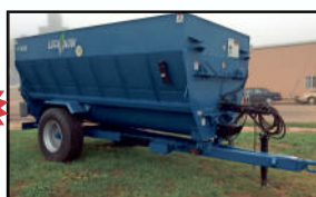
Luck Now XLR4410 Four Horizontal Augers With 410 Cubic FT. Capacity.
