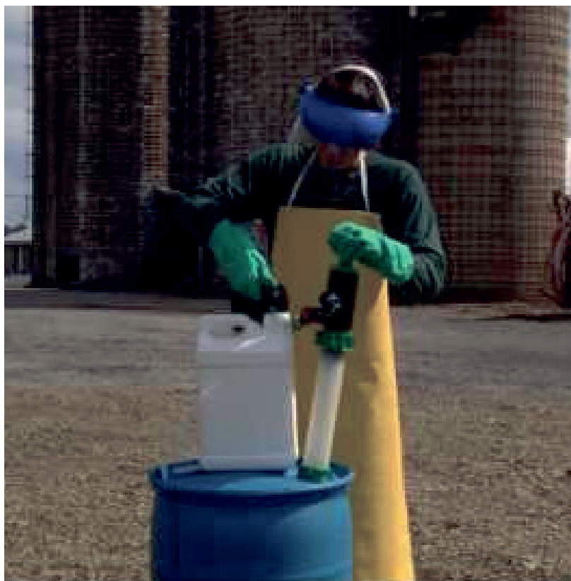
Using Closed and Sealed Systems for Loading and Mixing Plant Protection Products. Courtesy Photo
